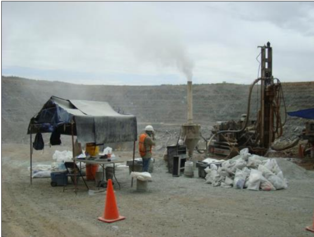
Figure 11.2 Reverse Circulation Sample Collection
