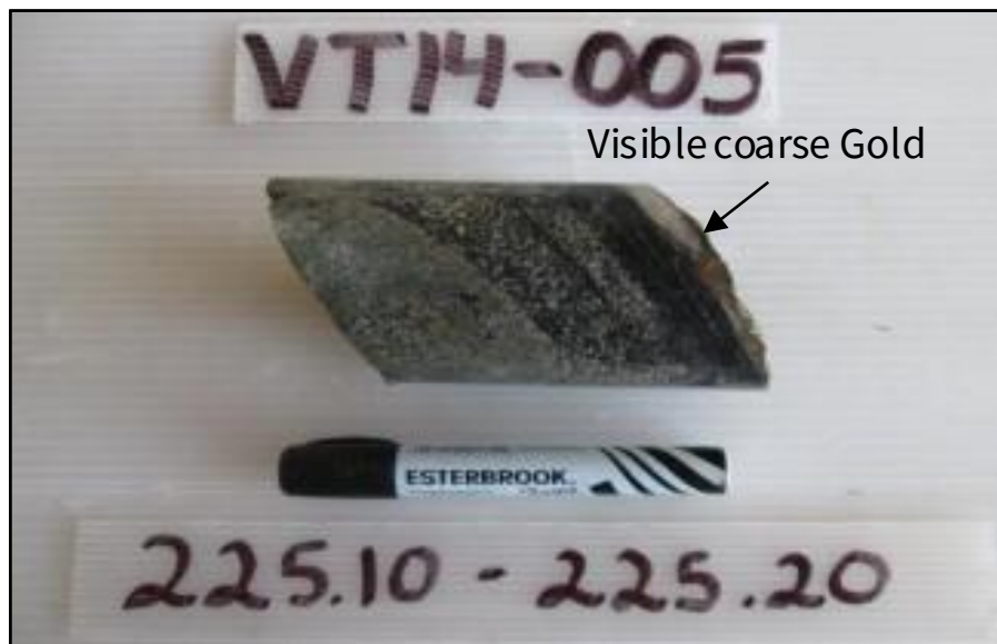
Figure 11.7 Drill Hole VT14-005 Showing a Location with Visible Gold in the Core
